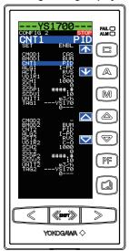
Operation Display > (sur) + (a) keys (to the Tuning Menu Display) > (sur) + (a) keys (to the Engineering Menu Display) > (CONFIG2) software key (Configuration Display 2)
