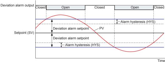
For an example in the figure above, the contact type is such that the contact opens if an event occurs (factory default).
