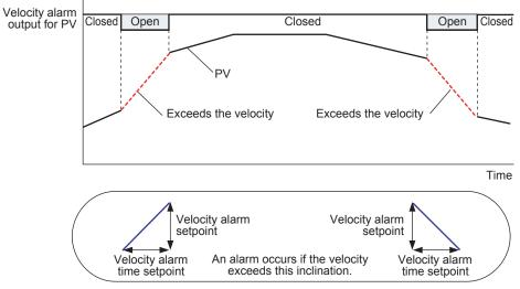
For an example in the figure above, the contact type is such that the contact opens if an event occurs (factory default).
