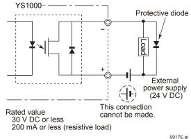
Figure 9.15 Connection Using Digital Output
