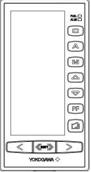
The operation mode can be switched by pressing the relevant key in the table below. This causes the light inside the key corresponding to the selected operation mode to light up. Note that on the ALARM Display, the operation mode cannot be switched.
