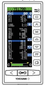
Operation Display >  $\P$  keys (to the Tuning Menu Display) > [PID1] software key (PID Setting Display 1) or [PID2] software key (PID Setting Display 2)
