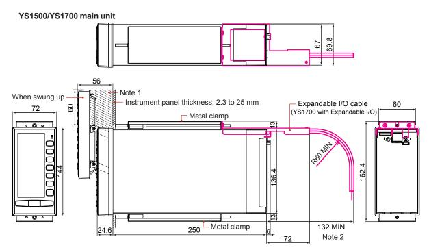
Weight: 1.6 kg (Basic type) 2.2 kg (Basic type with Expandable I/O)
