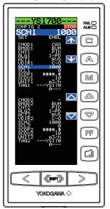
Operation Display > (serix) + (a) keys (to the Tuning Menu Display) > (serix) + (a) keys (to the Engineering Menu Display) > (CONFIG2) software key (Configuration Display 2)
