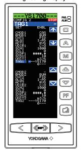
Operation Display > (Sur ) + (a) keys (to the Tuning Menu Display) > (Sur ) + (a) keys (to the Engineering Menu Display) > (CONFIG2) software key (Configuration Display 2)
