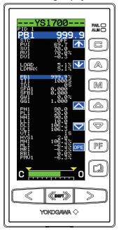
Operation Display > (Sur ) + (2) keys (to the Tuning Menu Display) > [PID1] software key (PID Setting Display 1) or [PID2] software key (PID Setting Display 2)
