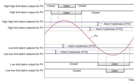
For an example in the figure above, the contact type is such that the contact opens if an event occurs (factory default).
