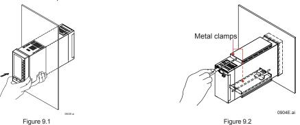
To remove the instrument from the panel, reverse the above procedure.
