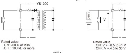
Figure 9.13 Connection of Digital Input (No-voltage Contact)
