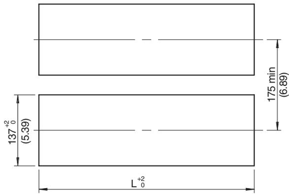
Side-by-side Mounting (vertically, max. 3 units)
