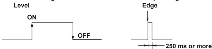
For contact inputs, the remote signal rises when the contact switches from open to closed and falls when the contact switches from closed to open. For open collector signals, the remote signal rises when the collector signal (voltage level of the remote terminal) goes from high to low and falls when the collector signal goes low to high. You can reverse the above operations (see section 7.3 for details).
