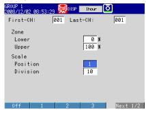
Number of Displayed Scale Digits and Current Value Indicator Press MENU (to switch to setting mode), and select the Menu tab > Display > Trend.
