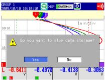
Select Yes using the arrow keys and press DISP/ENTER. On models with the computation function (/M1 or /PM1 option), select Mem+Math or Memory, and press DISP/ENTER.
