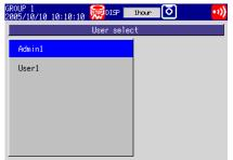
**2.** Press the **arrow keys** to select a user name, and press **DISP/ENTER**. A window appears for you to enter the password.
