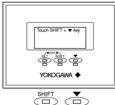
Touch SHIFT and ▼ switches simultaneously.
