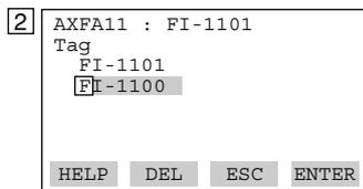
The display for the Tag setting appears. (The default value of “Tag” is blank.)
