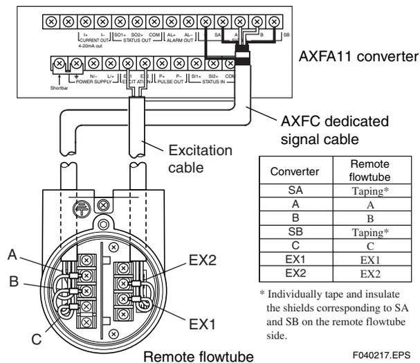
Figure 4.4.7 Wiring Diagram
