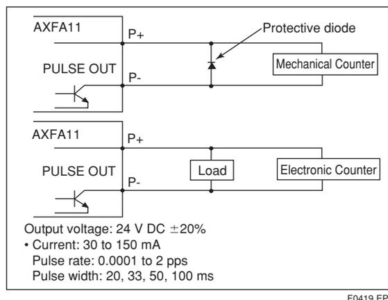
Figure 4.4.11 Active Pulse Output Connection (Optional code EM)
