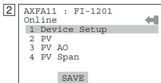
Select the desired field device. After that, normal communication with the selected field device is possible. The communication speed, however, is slow in this case.
