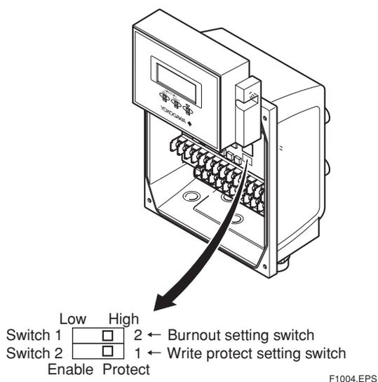
Figure 10.2.2 Switch Configuration
