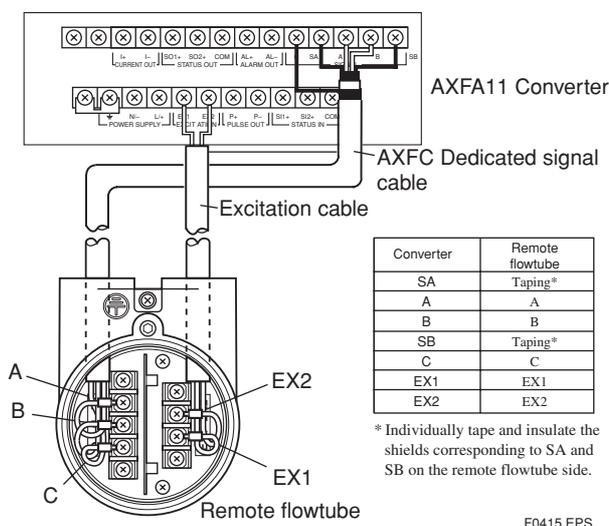
Figure 4.4.5 Wiring Diagram
