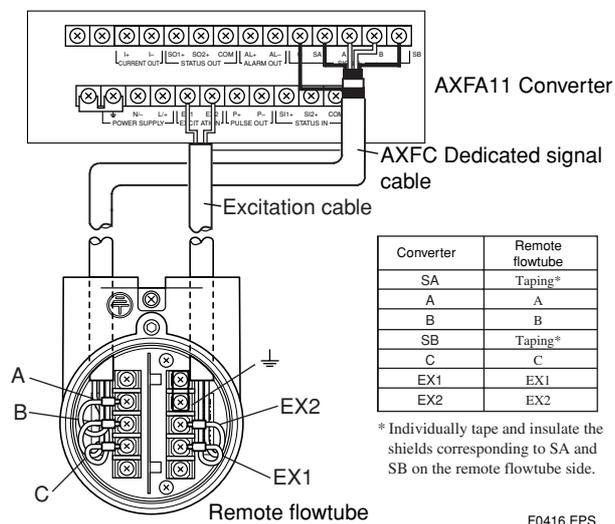
Figure 4.4.6 Wiring Diagram
