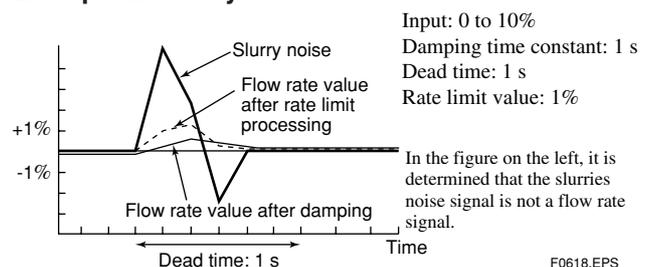
In the figure on the left, it is determined that the slurries noise signal is not a flow rate signal.
