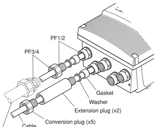
When working on electric wire tube or flexible tube (PF3/4)
