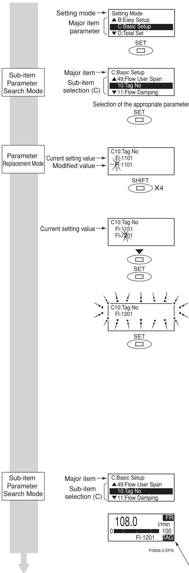
The cursor has been moved to **C: Basic Setup** in this screen.
