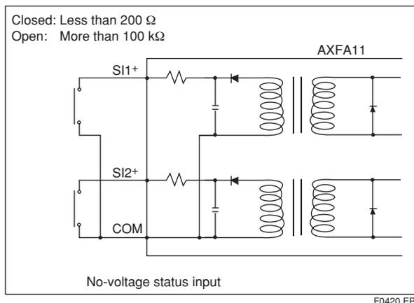
Figure 4.4.12 Status Input Connection
