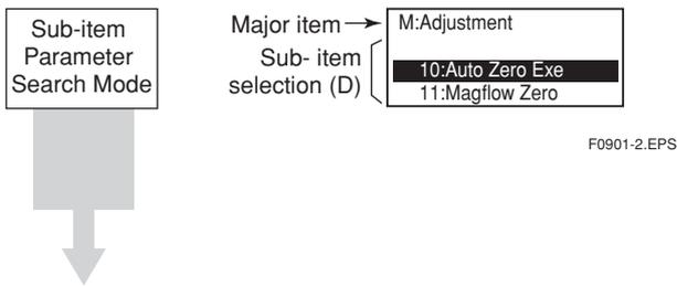
When zero adjustment function has been completed, the system automatically returns to the sub-item selection screen (D).
