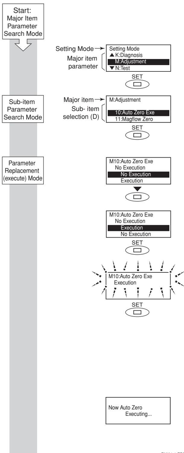
Once in Setting Mode, use the switch to move the cursor to **M: Adjustment**.
