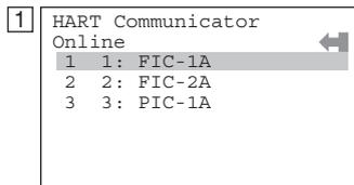
The HART Communicator searches for field devices that are set in the multidrop mode when the HART Communicator is turned on.
